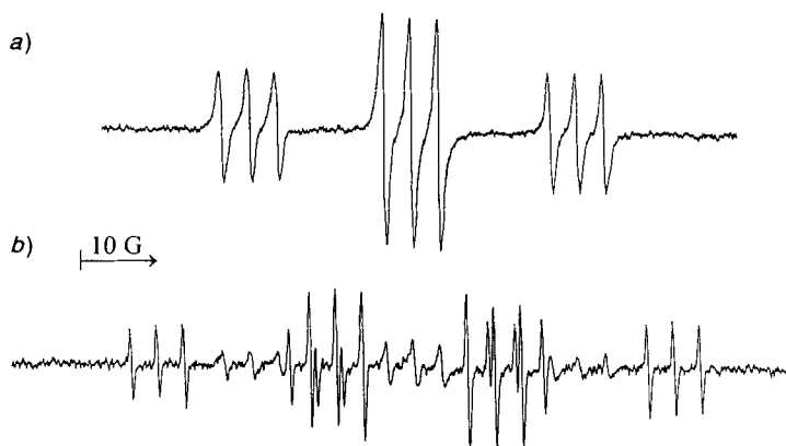
Fig. 1. ESR Spectra obtained during photolysis of dibenzoyl peroxide in acetonitrile; a) in the absence of alkenes, b) in the presence of 0.03 M acrylonitrile
